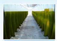
Algae plant CO<sub>2</sub> binding by microalgae (pilot plant; since 2008)
